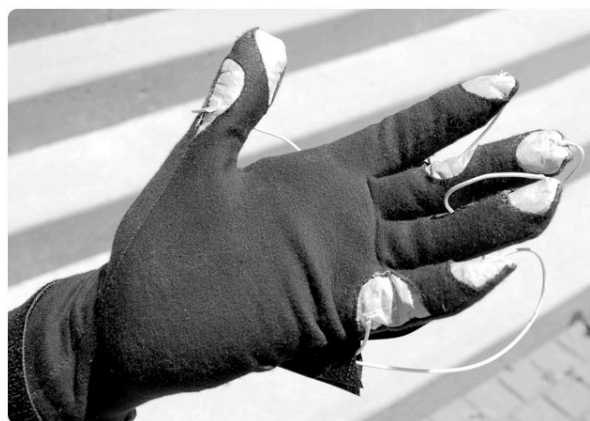
Figure 2: Contact surfaces on the TouchGlove.
