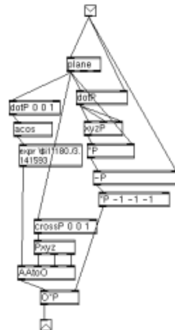
Figure 2: Typical example of geometric computing using the new Max/FTS position and orientation objects. This Max patcher takes a list of positions , projects these on the plane that best fits them, then rotates the plane (with projected positions ) and eliminates z. This patcher enables subsequent fitting of 2-D parametric curves to the x-y coordinates (e.g. the x-y coordinates computed from the positions marking the thumb and index fingers).
