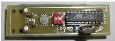
Figure 4. Top view of the IR tag with two LEDs
